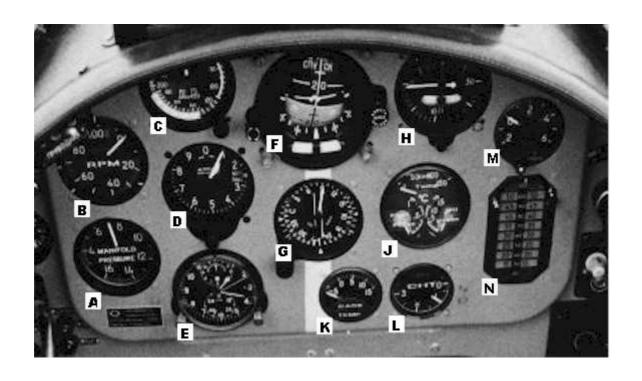
Manifold Pressure (in cms of Hg) Α RPM in percent В C Airspeed Indicator D Altimiter Ε Clock / Stop watch / Timer F Attitude Indicator G Gyro Compass / ADF / RMI Н Turn & Bank / Rate of Climb Indicator Oil Temp, Oil Pressure, Fuel Pressure J K Carb. Inlet Temperature Cylinder Head Temperature L Voltmeter / Ammeter M Digital Fuel Gauge Ν
