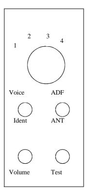
The TEST switch causes the instrument pointer to rotate around the dial. The ADF/Antenna switch selects normal Radio compass operation (ADF) or audio only (Antenna) The Voice/Ident switch selects the Morse code ident from the NDB or its voice transmission.
