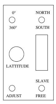
The Gyro compass installed in the Yak 52 is a slaved gyro with latitude compensation. It may be operated in a slaved or free mode.
